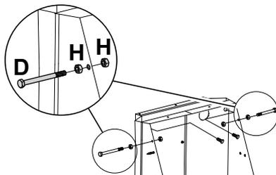
8. The stand will need to be secured on the floor through the holes located at the base of the stand.
