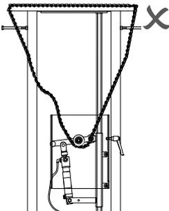
7. If the chain tension is too loose, repeat the procedure.
