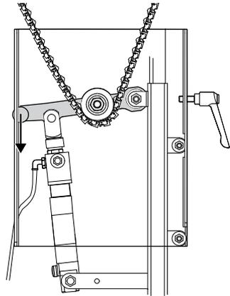
4. Move the tensioner downward until the chain is tightly secured in its position. There should be a gap of about 10–15 mm between the pneumatic-piston nut and pneumatic piston, where the piston should be visible.
