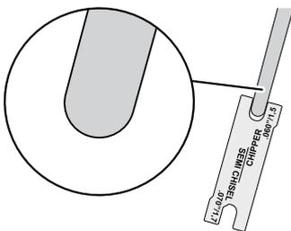
8. Repeat steps 4–8 until the grinding wheel profile is the same as the selected profile on the profile template.
