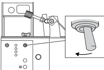
3. Set the chain pusher switch to ON to start the feeding of the chain and the movement of the grinding head. The sharpening will start after this.
