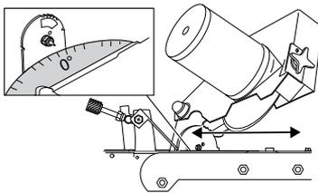
4. Set the head tilt angle to 60°. (See 3.6.1, "Grinding speed knob")
