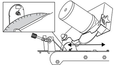
3. Tighten the head-tilt angle nut.
