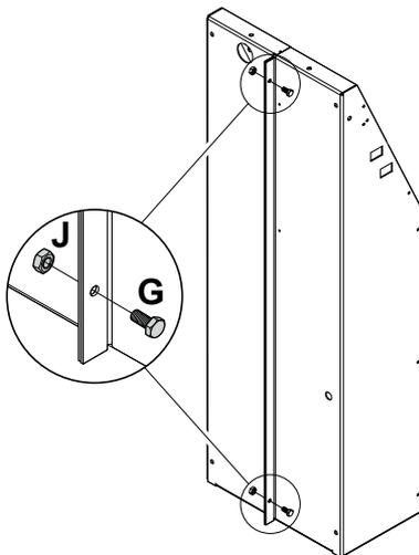
3. To complete the assembly of the stand, bolt the side support first to the base and then to the front piece.
