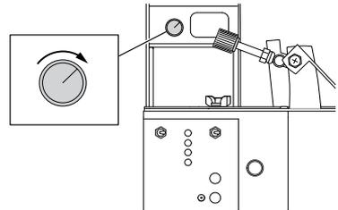
3. Set the grinding wheel switch to ON.
