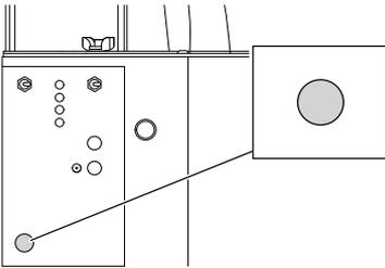
2. Lift the grinding head to its most upright position.
