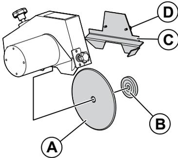
3. Remove the wheel attachment nut from the hub.
