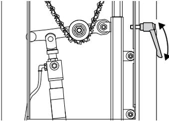
6. Gently press the chain with your hand to test the tension. The chain should not slacken.
