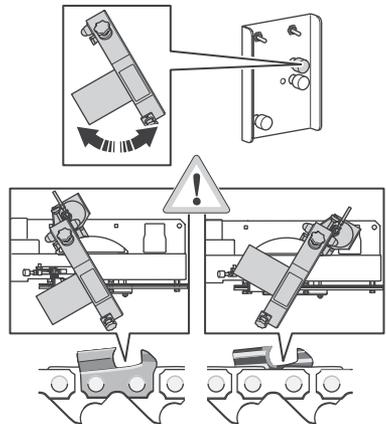
3. Lift the grinding head to its uppermost position.
