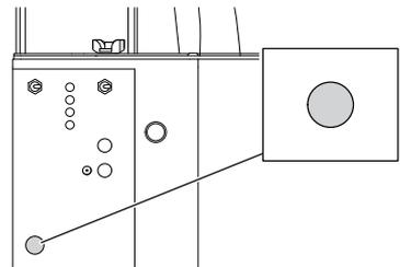
**IMPORTANT** Grinding dust can interfere with the machine's operation. Clean the machine daily to remove all of the grinding dust. Use a vacuum cleaner, brush or similar to clean the machine.
