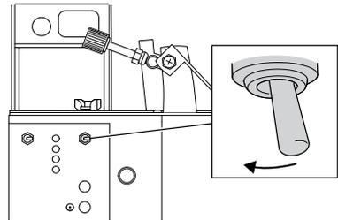
4. Make sure that the grinding wheel does not vibrate or wobble. If the grinding wheel is damaged, it must be replaced immediately; see 6.3, "Change the grinding wheel and fit the grinding wheel guard".
