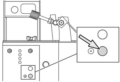
2. Set the grinding speed knob to medium speed.
