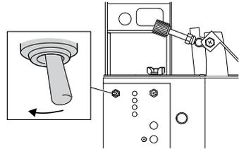
4. Press the reset button when the grinding head moves downward the first time. This resets the counter.
