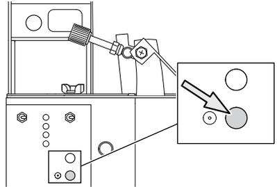
2. Press the grinding head positioning button to move the grinding head so that it is tilted in the correct start position for the next cutting link to be ground.
