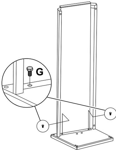
2. Next, attach the two side pieces to each other with provided bolts through the holes at the intersection of two pieces to create the side support piece.
