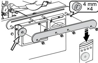
3. Replace the 4 mm distances with the 2,5 mm distances that can be found in the packing material for the machine.
