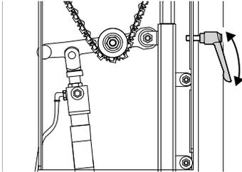
2. Lift the tensioner arm (there is a quick release function) and place the chain below the tensioner roll.
