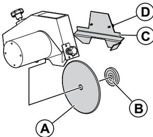
5. Remove the grinding wheel (A) from the grinding wheel axis and discard it in accordance with local, state and national laws and regulations.
