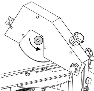
4. Next, insert the appropriate wheel onto the hub and, using moderate pressure with your hands, secure the wheel attachment nut to hold the wheel in place.
