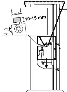
5. Tighten the locking handle to secure the chain.
